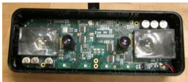
Inside of nano NXT camera are 2 cameras and IR LED illuminators.
